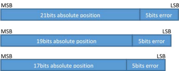
Figure 9: AR18 SSI 3-Wire Format Output
