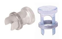
The slotted screw with knurled nut provides effective shield bonding of large aircore and filled service wires up to ½" shield O.D. (11, 16 and 25 pairs) to a ground wire or ground stud. Can also be used to bond the two pieces of butt spliced service drop within a buried service drop closure.
