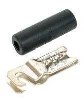
The one-piece clip, bonds or grounds the shield of a service wire or small cable up to ¼" O.D. or 3/8" O.D. at station protectors, pedestals and similar terminations. Low resistance path to ground prevents stray electromagnetic interference from inducing noise or cross talk on cable pairs and provides a ground circuit path from the shield to the ground protector.
