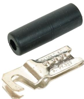
The one-piece clip, bonds or grounds the shield of a service wire or small cable up to  $\frac{1}{4}$ ” O.D. or  $\frac{3}{8}$ ” O.D. at station protectors, pedestals and similar terminations. Low resistance path to ground prevents stray electromagnetic interference from inducing noise or cross talk on cable pairs and provides a ground circuit path from the shield to the ground protector.
