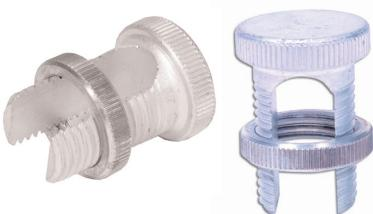
The slotted screw with knurled nut provides effective shield bonding of large aircore and filled service wires up to  $\frac{1}{2}$ ” shield O.D. (11, 16 and 25 pairs) to a ground wire or ground stud. Can also be used to bond the two pieces of butt spliced service drop within a buried service drop closure.
