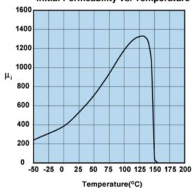
Measured on a 17/10/6mm toroid at 100kHz.
