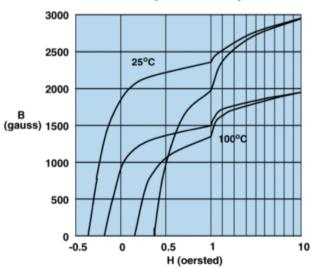
Measured on a 17/10/6mm toroid at 10kHz.
