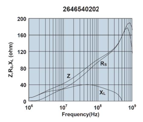
Impedance, reactance, and resistance vs. frequency.
