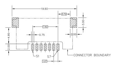
RECOMMENDED MOUNTING LAYOUT RECOMMENDED PCB T: 1.6mm TOLERANCE UNLESS OTHERWISE ±0.1mm
