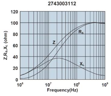
Impedance, reactance, and resistance vs. frequency.
