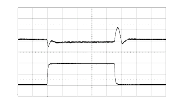
Output Load Transient Response, Default PID/NLR
