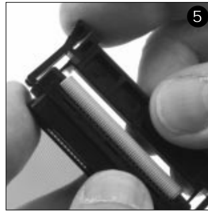
The 101XX-8000 plug may be assembled with a strain relief that is installed on the topside of the plug. Bend cable over the top of the connector and snap both inside and outside latches into the body.
