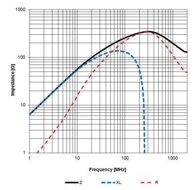
Test Equipment: E4991A or equivalent
