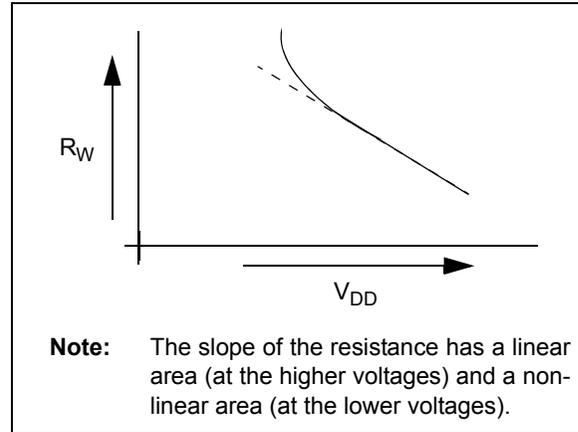
**FIGURE 6-4:** Relationship of Wiper Resistance ( $R_W$ ) to Voltage
