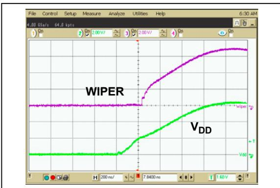
**FIGURE 2-14:** 2.1 kΩ – Power-Up Wiper Response Time.
