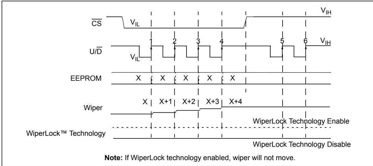
**FIGURE 5-1:** Increment without Writing Wiper Setting to EEPROM.
