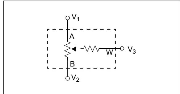
**FIGURE 6-3:** Potentiometer Configuration.
