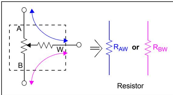
**FIGURE 6-2:** Rheostat Configuration.
