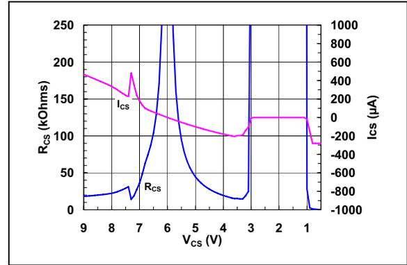
**FIGURE 2-4:**  $\overline{\text{CS}}$  Pull-up/Pull-down Resistance ( $R_{CS}$ ) and Current ( $I_{CS}$ ) vs.  $\overline{\text{CS}}$  Input Voltage ( $V_{CS}$ ) ( $V_{DD} = 5.5\text{V}$ ).
