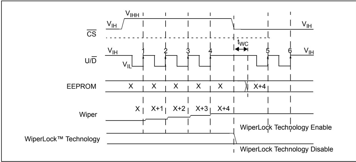
**FIGURE 5-6:** High-Voltage Increment and Disable WiperLock™ Technology.
