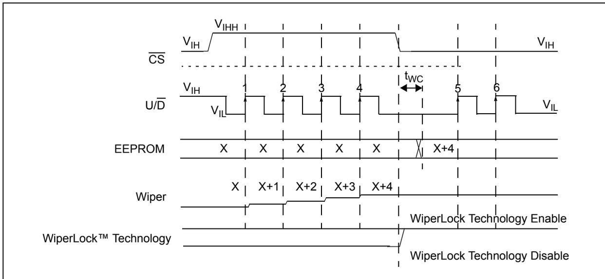
**FIGURE 5-7:** High-Voltage Increment and Enable WiperLock™ Technology.
