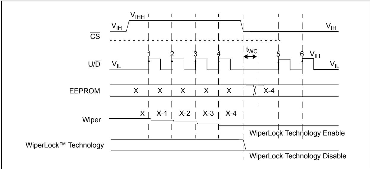
**FIGURE 5-8:** High-Voltage Decrement and Disable WiperLock™ Technology.
