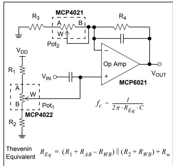
**FIGURE 8-5:** Programmable Filter.
