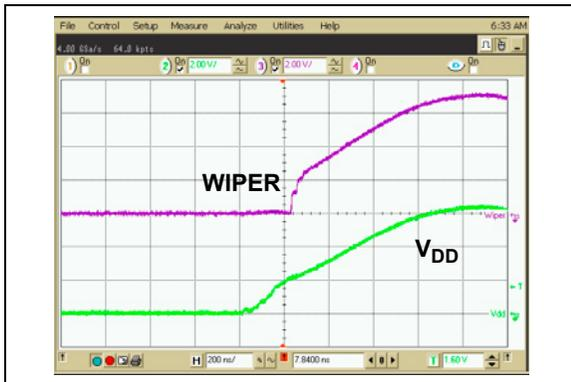
**FIGURE 2-45:**  $50\text{ k}\Omega$  – Power-Up Wiper Response Time.
