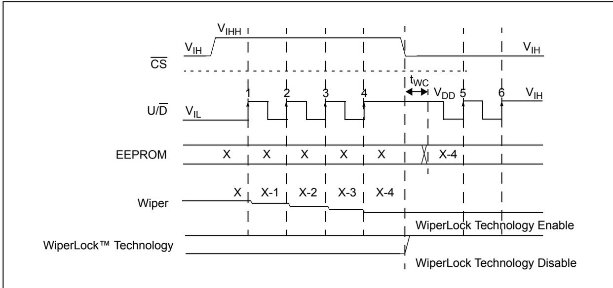
**FIGURE 5-9:** High-Voltage Decrement and Enable WiperLock™ Technology.
