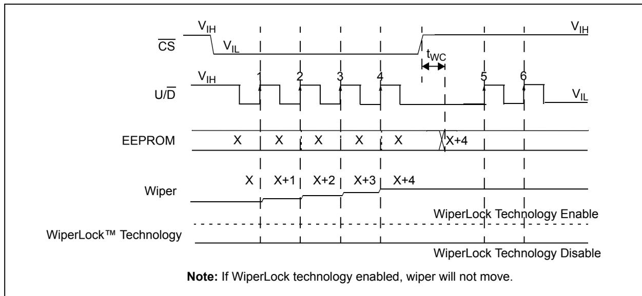
**FIGURE 5-2:** Increment with Writing Wiper Setting to EEPROM.
