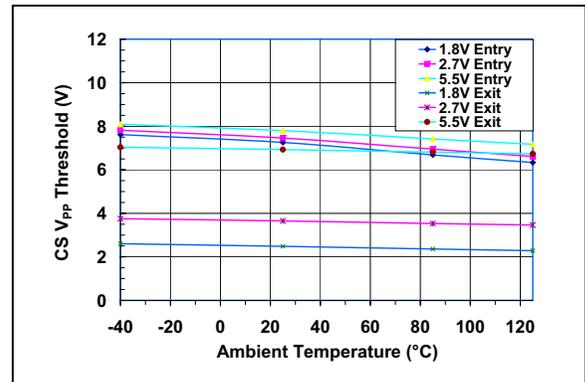
**FIGURE 2-5:**  $\overline{\text{CS}}$  High Input Entry/Exit Threshold vs. Ambient Temperature and  $V_{DD}$ .
