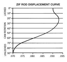
The ZIF cam detent design gives added assurance that a PCB will remain securely locked in position even under extreme vibration and shock levels. Detent action occurs during the final 15 degrees of cam rotation and virtually eliminates any possibility of the cam unlocking under environmental stress.
