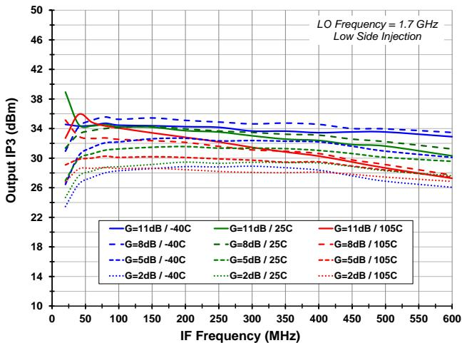
**Figure 26. Output IP3 vs. Temperature and Gain Setting (LO=2.25 Ghz)**
