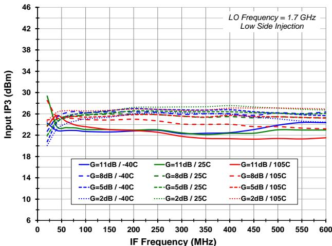
**Figure 22. Input IP3 vs. Temperature and Gain Setting (LO=2.25 Ghz)**
