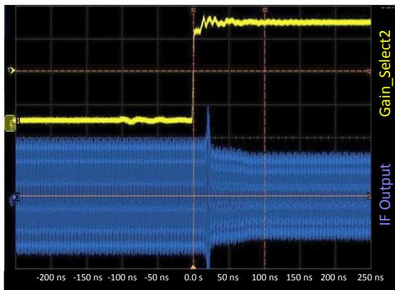
**Figure 49. Gain Settling Time for 5 dB to 8 dB Gain Setting**
