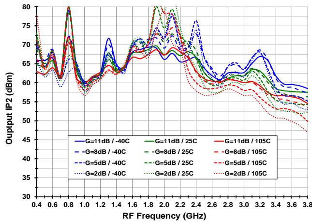
**Figure 18. Output IP2 vs. Temperature and Gain Setting (Vcc = 3.15, Tcase = 105C)**
