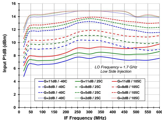
**Figure 34. Input P1dB vs. Temperature and Gain Setting (LO=2.25 Ghz)**
