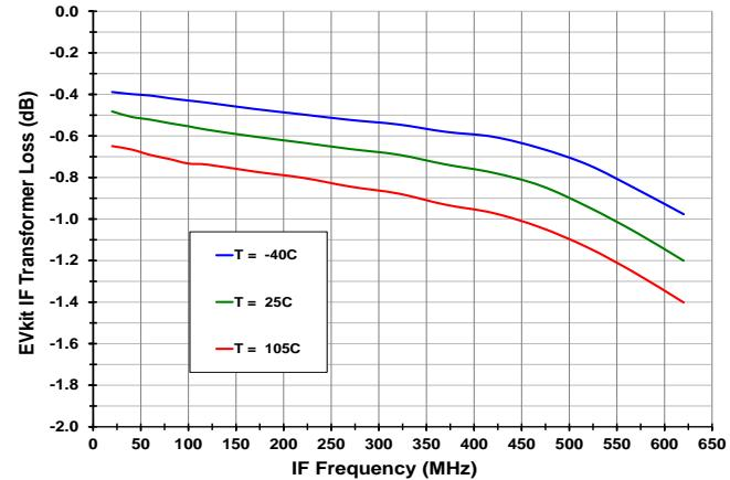
**Figure 44. Evaluation Kit RF Trace Loss vs. Temperature**
