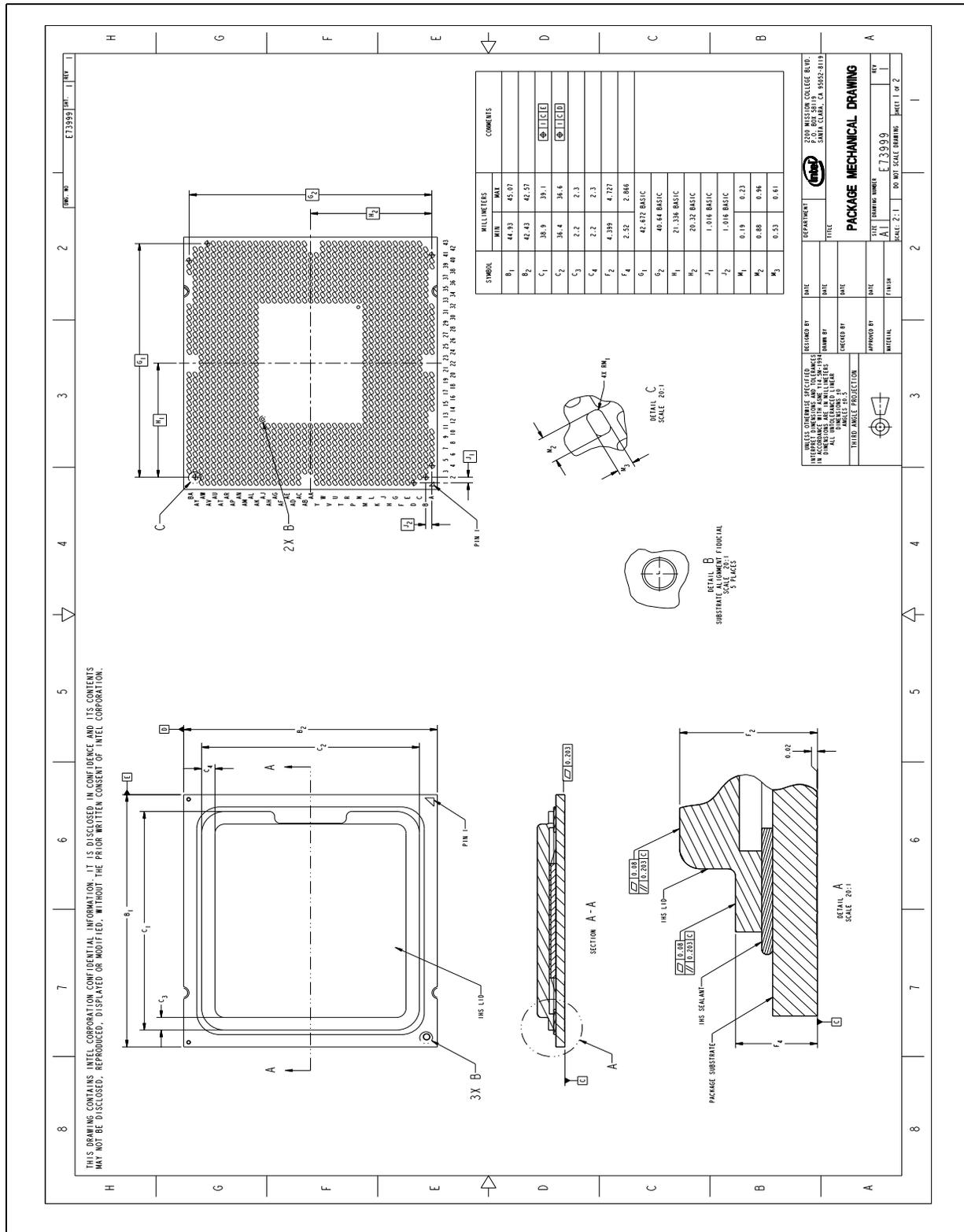
Figure 9-3. Processor Package Drawing Sheet 2 of 2
