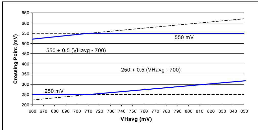
Figure 7-7. BCLK{0/1} Differential Clock Measurement Point for Ringback
