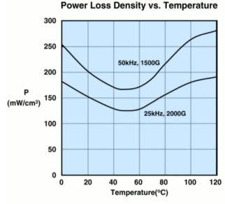
Measured on an 18/10/6mm toroid using the Clarke Hess 258 VAW.
