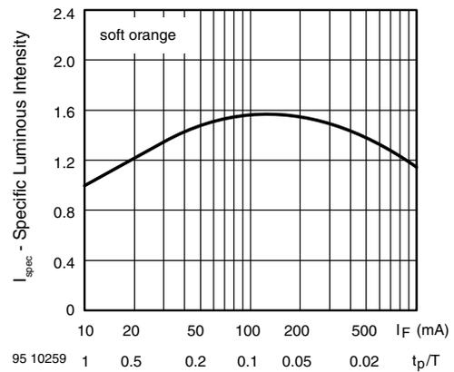
Fig. 8 - Relative Luminous Intensity vs. Forward Current/Duty Cycle
