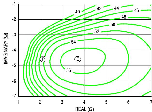
Figure 17. P1dB Load Pull Fficiency Contours (%)
