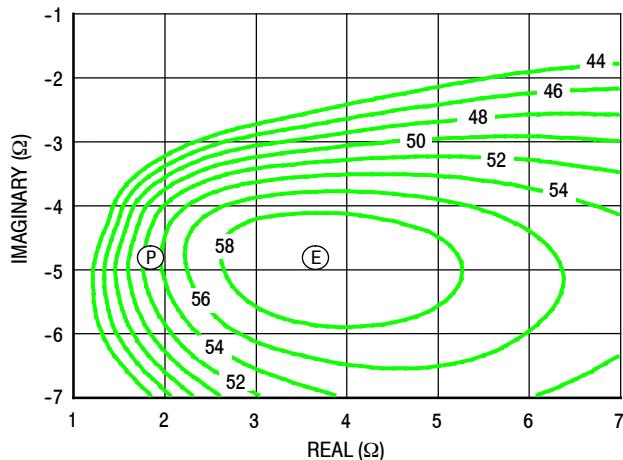
Figure 21. P3dB Load Pull Fficiency Contours (%)
