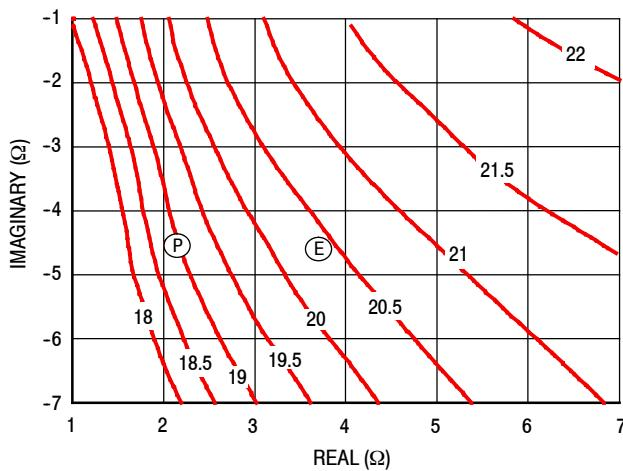
Figure 18. P1dB Load Pull Gain Contours (dB)
