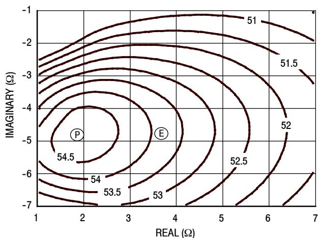
Figure 20. P3dB Load Pull Output Power Contours (dBm)
