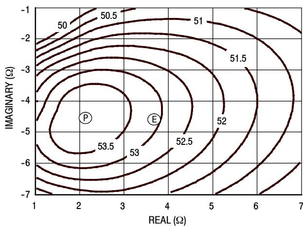
Figure 16. P1dB Load Pull Output Power Contours (dBm)
