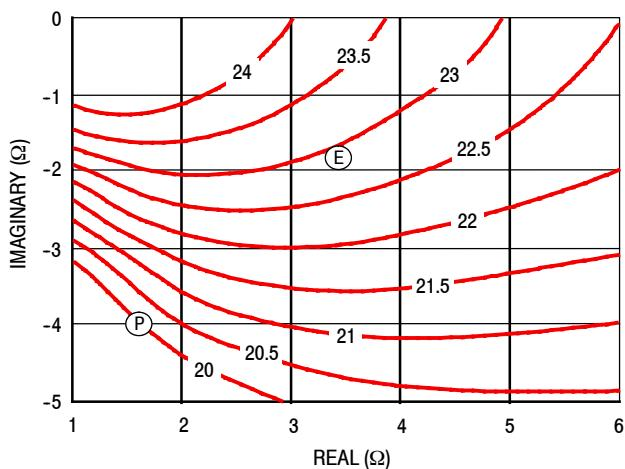
Figure 10. P1dB Load Pull Gain Contours (dB)
