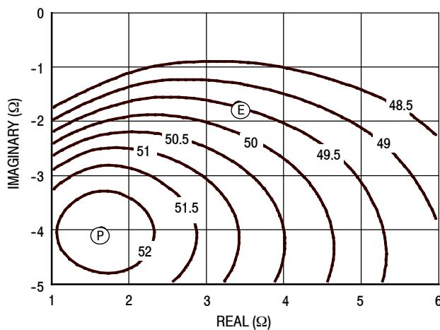
Figure 12. P3dB Load Pull Output Power Contours (dBm)
