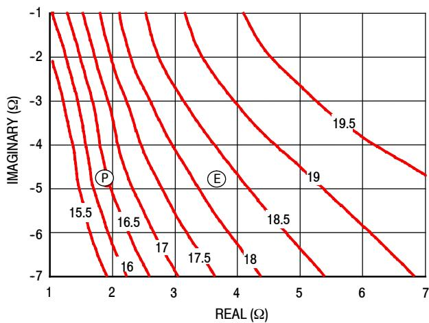
Figure 22. P3dB Load Pull Gain Contours (dB)
