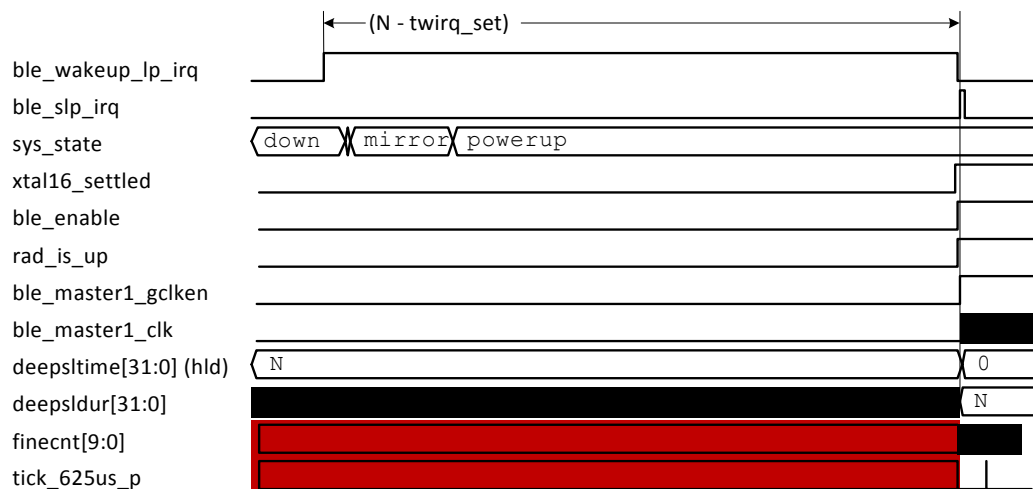
Figure 64 Exit BLE Deep Sleep Mode at Predetermined Time (Zoom Out)
