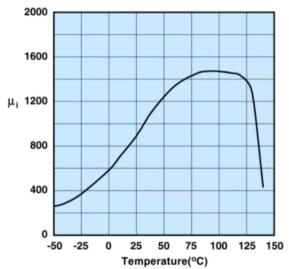
Measured on a 17/10/6mm toroid at 100kHz.
