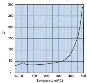
Measured on a 19/10/6mm toroid at 100 kHz.
