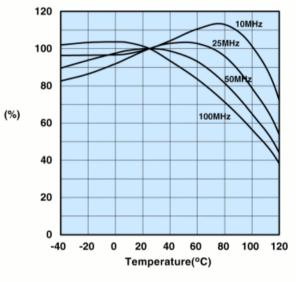
Measured on a 2631000301 using the HP4291A.
