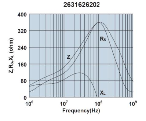
Impedance, reactance, and resistance vs. frequency.
