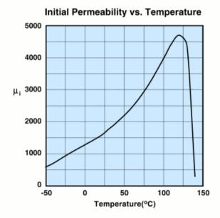
Measured on a 17/10/6mm toroid at 100kHz.
