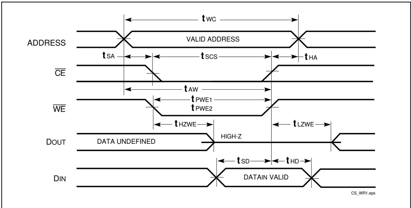
WRITE CYCLE NO. 2 ( $\overline{OE}$  is HIGH During Write Cycle) <sup>(1,2)</sup>
