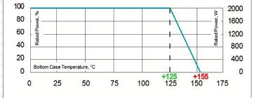
Derating (thermal resist.)FPA2K: 66.6 W/K (0.015K/W) Power Rating:2000 W at 125°C bottom case temperture.
