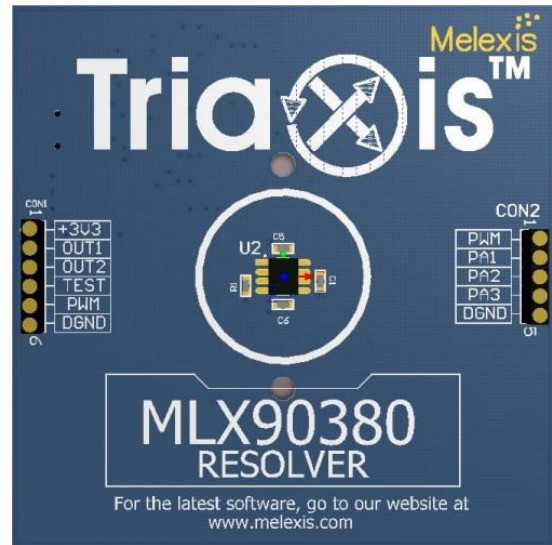
Figure 1: MLX90380 Resolver Evaluation/Demonstration board
