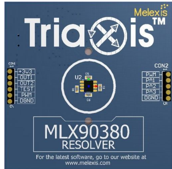
Figure 1: MLX90380 Resolver Evaluation/Demonstration board
