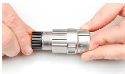
Step 15 - Push sub-assembly into shell
