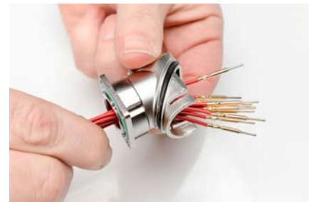
Step 4 - Crimp contacts onto wire
