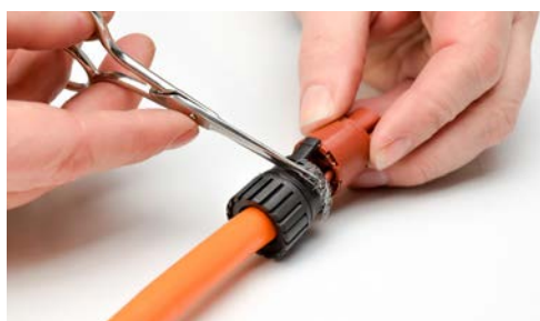
Step 14 - Trim shield as shown
