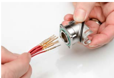
Step 3 - Slide wires through shell
