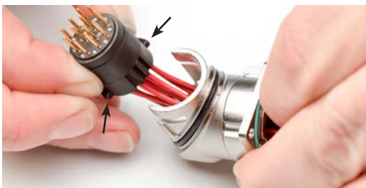
Step 5 - Locate keys on sides of insert
