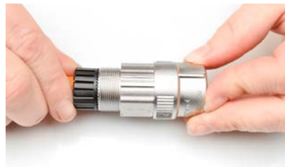
Step 15 - Push sub-assembly into shell
