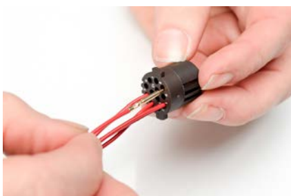
Step 4 - Push wire into insert
