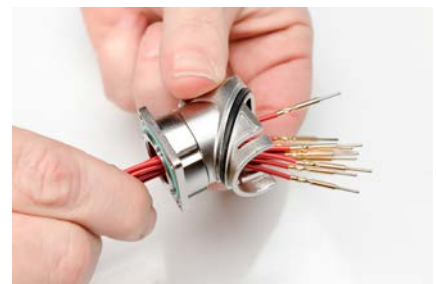
Step 4 - Crimp contacts onto wire
