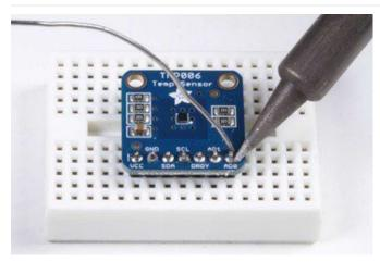
And Solder! Solder each pin for a solid electrical connection.
