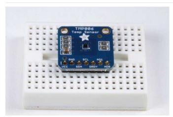
Position the Breakout Place the breakout board over the short end of the header pins.
