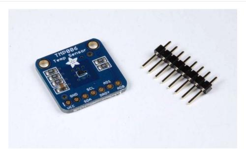
The TMP006 Thermopile Breakout comes with all surface-mount components pre-soldered. For use on a breadboard you will want to solder in the supplied header.
