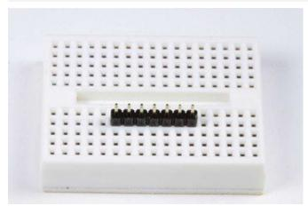
Position the Header Cut the header to length and insert it in a breadboard with the long pins down.
