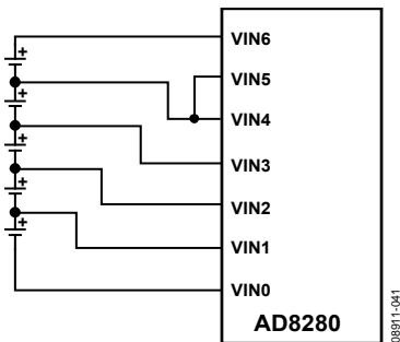
Figure 47. Five-Cell Connections for the AD8280
