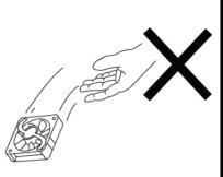
Don't cut the fan or lead wires
