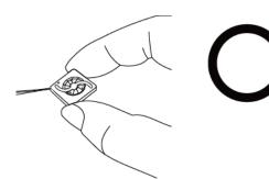
Don't pull fan with lead wires.
