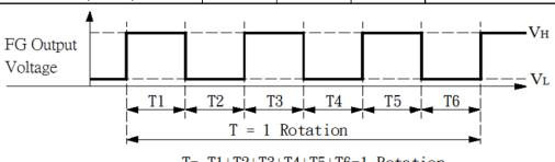
T= T1+T2+T3+T4+T5+T6=1 Rotation  $T = \frac{60}{rpm}$
