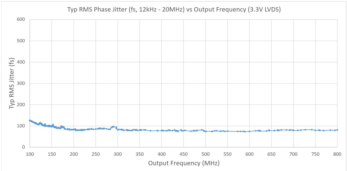
Phase jitter measured with Agilent E5052 using a differential-to-single ended converter (balun or buffer). Measurements collected for >700 commonly used frequencies. Phase noise plots for specific frequencies are available using our free, online Oscillator Phase Noise Lookup Tool at [www.silabs.com/oscillators](http://www.silabs.com/oscillators).
