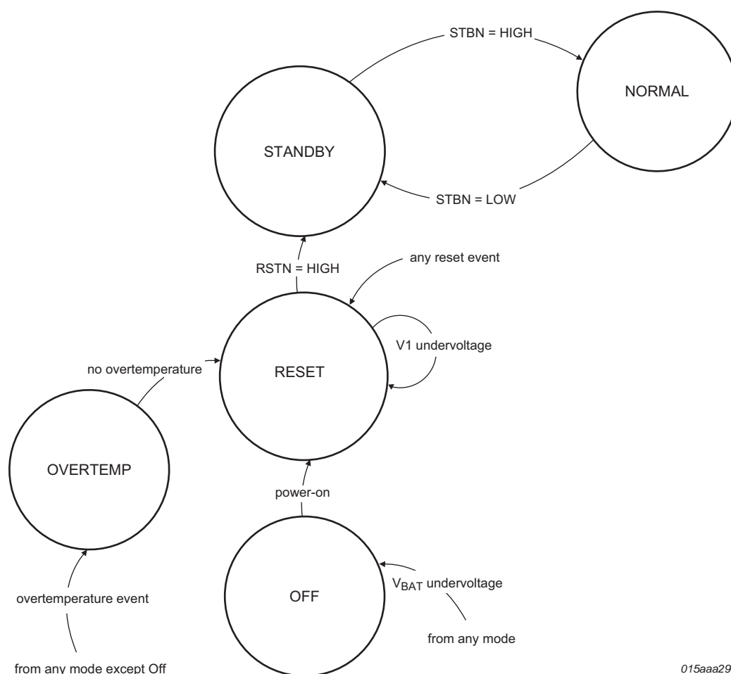
Fig 3. UJA1163 system controller state diagram
