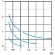
**DC-** Control of electromagnets (L/R  $\leq$  2 x (Ue x le) in ms, with Ue: rated operating voltage and le: rated operating current) 13
