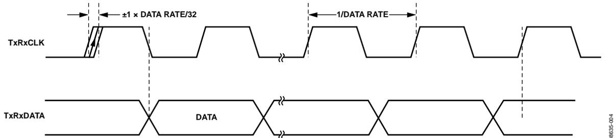
Figure 4. TxRxDATA/TxRxCLK Timing Diagram in Receive Mode
