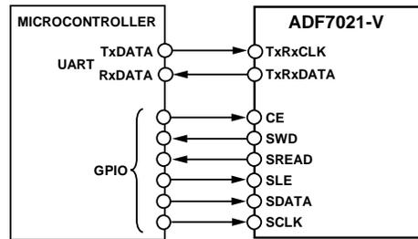
Figure 59. ADF7021-V (UART Mode) to Asynchronous Microcontroller Interface
