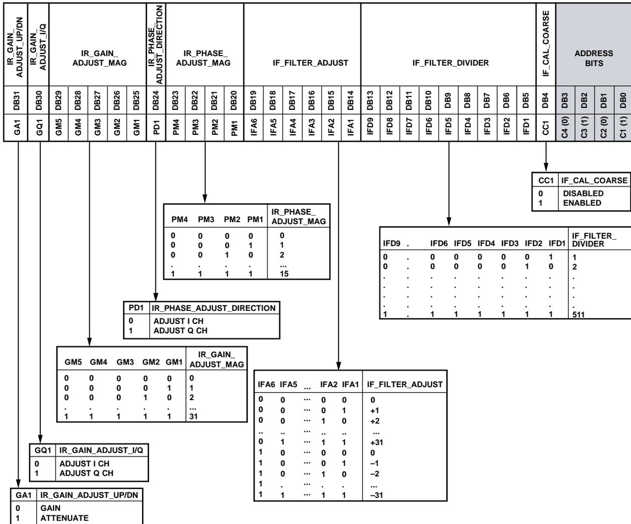
Figure 67. Register 5—IF Filter Setup Register Map
