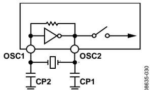
Figure 32. Crystal Oscillator Circuit on the ADF7021-V
