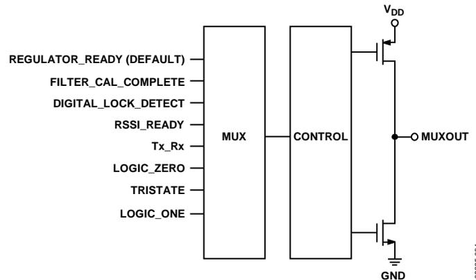
Figure 36. MUXOUT Circuit
