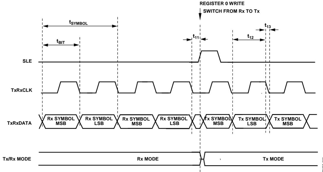
Figure 6. Receive-to-Transmit Timing Diagram in 4FSK Mode
