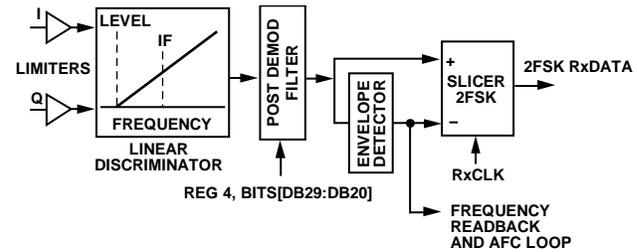
Figure 48. Block Diagram of Linear FSK Demodulator
