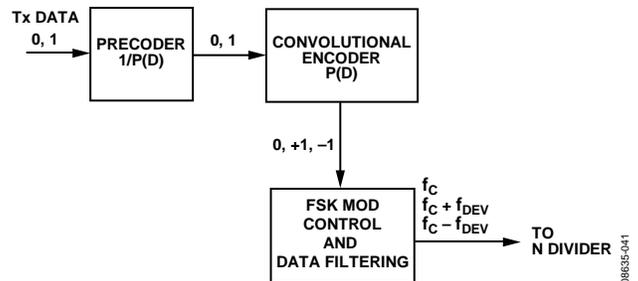
Figure 42. 3FSK Encoding
