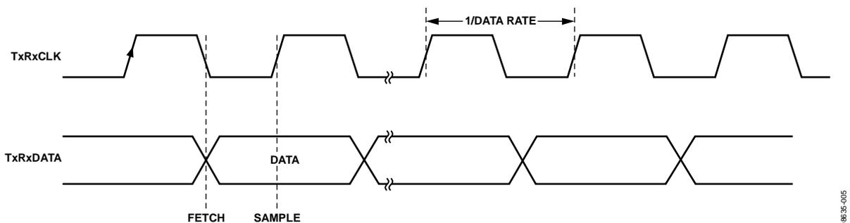
Figure 5. TxRxDATA/TxRxCLK Timing Diagram in Transmit Mode
