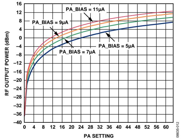
Figure 14. RF Output Power vs. PA Setting
