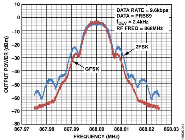
Figure 16. Output Spectrum in 2FSK and GFSK Modes
