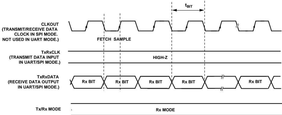
Figure 9. Receive Timing Diagram in UART/SPI Mode
