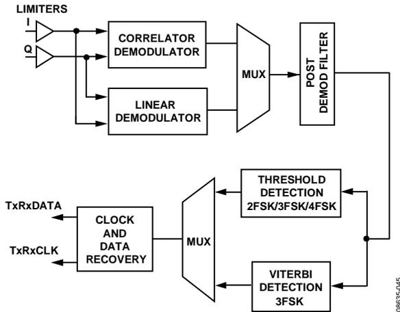
Figure 46. Overview of Demodulation, Detection, and CDR Process
