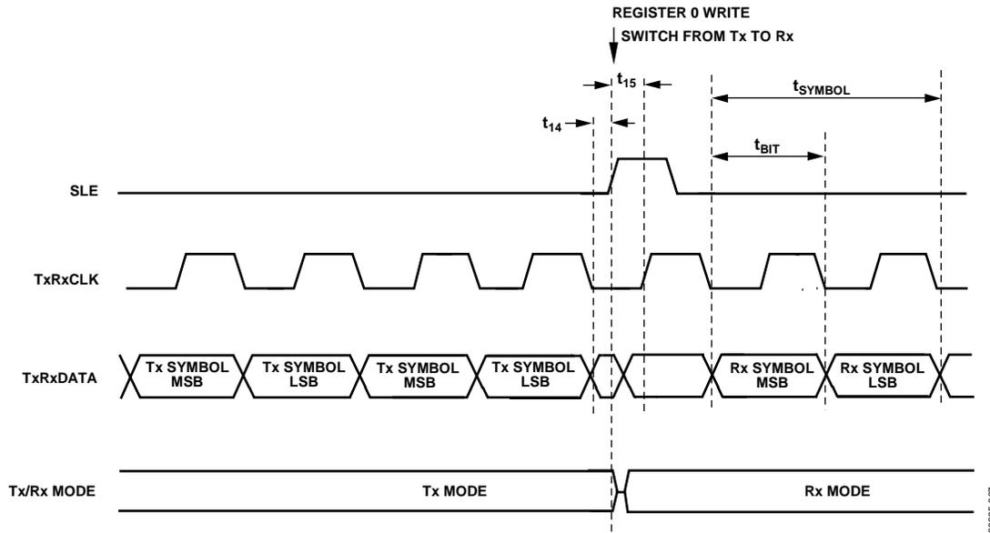
Figure 7. Transmit-to-Receive Timing Diagram in 4FSK Mode
