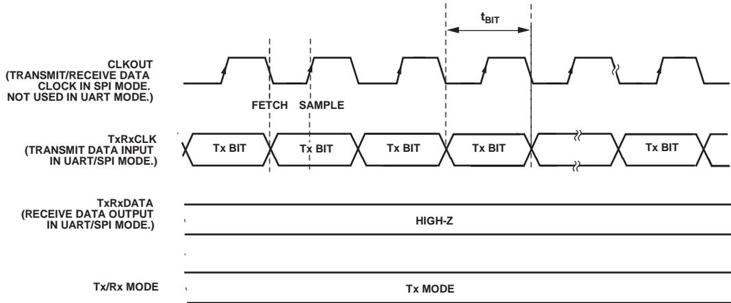
Figure 8. Transmit Timing Diagram in UART/SPI Mode
