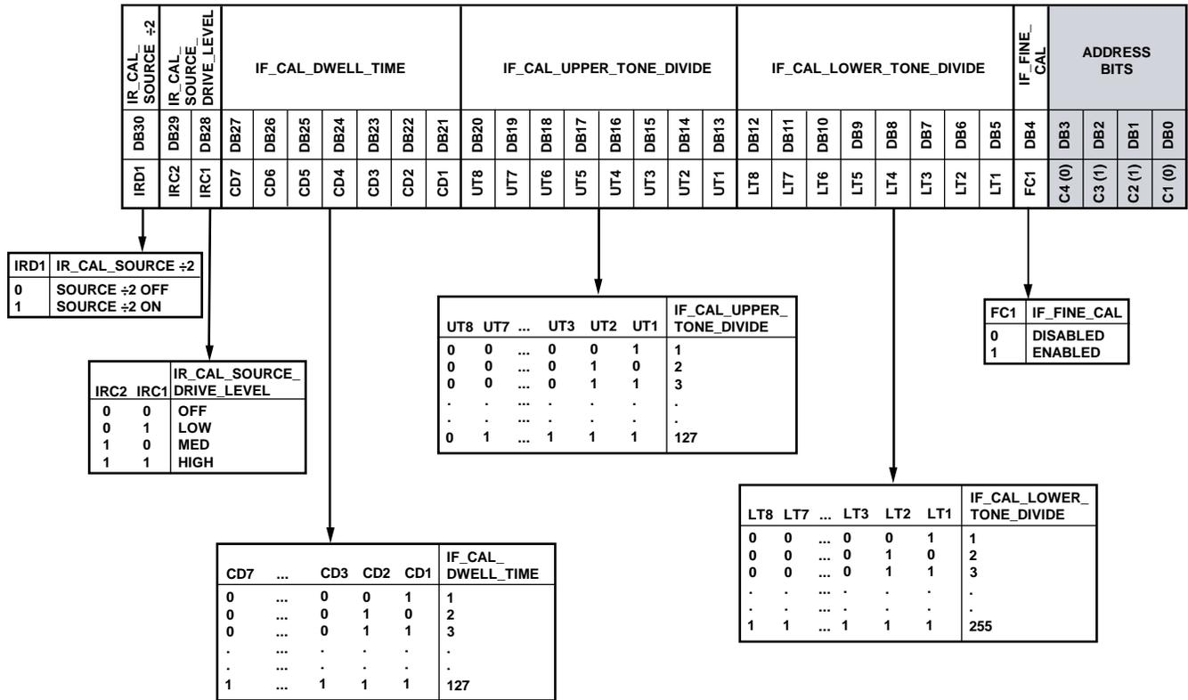
Figure 68. Register 6—IF Fine Calibration Setup Register Map
