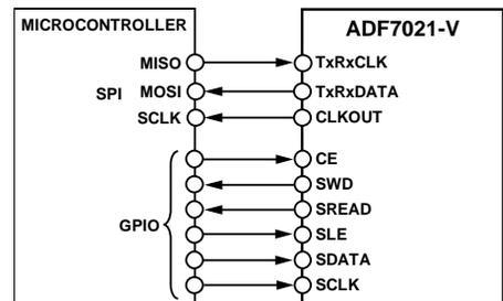
Figure 60. ADF7021-V (SPI Mode) to Microcontroller Interface
