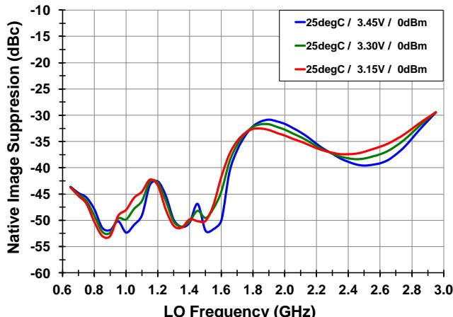
**Unadjusted LO Suppression vs.  $V_{CC}$**
