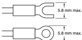
Use wires that withstand a minimum of 70°C.
