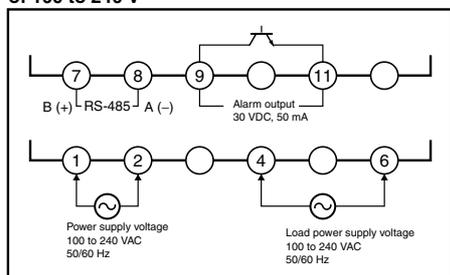
Note: Connect the power supply (100 to 240 VAC) for the G3ZA across terminals 1 and 2 and the load power supply for the SSR loads across terminals 4 and 6.
