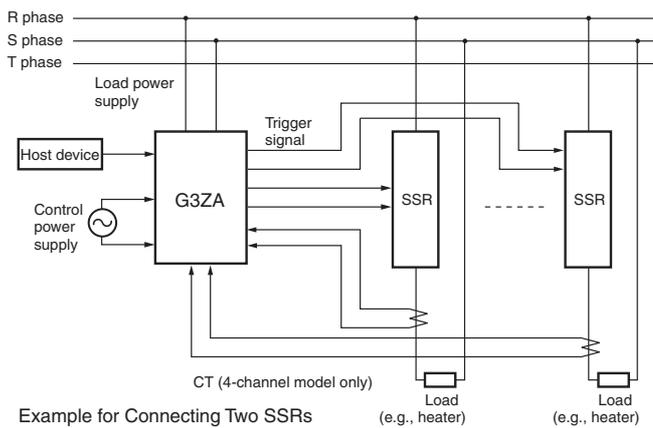
**Note:** Connect a power supply with the same phase as the SSRs to the load power supply terminals on the G3ZA.
