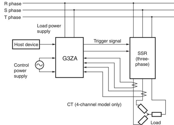
**Note:** Connect to one of the three phases on the load power supply input terminals of the G3ZA.
