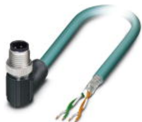
Assembled Ethernet cable, CAT5e, shielded, 2-pair, 26 AWG stranded (7-wire), RAL 5021 (water blue), angled M12 plug to free cable end, line, length: 1.5 m
