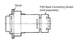
Note: The mounting panel thickness should be 1 to 5 mm.
