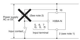
**Note: 1.** Power supply terminal 2 is a common terminal for the input signals (G, S, R) to the Timer. Never use terminal 10 as the common terminal for this purpose, otherwise the internal circuit of the Timer may be damaged.
