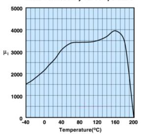
Measured on a 17/10/6mm toroid at 10kHz.
