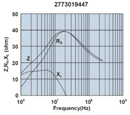
Impedance, reactance, and resistance vs. frequency.
