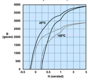
Measured on a 17/10/6mm toroid at 10kHz.
