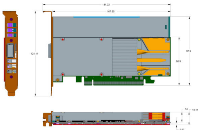
Figure 4. Acceleration Card - Standard Profile Bracket with Airduct
