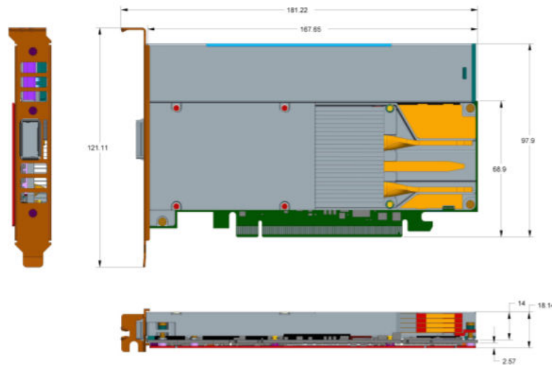
Figure 4. Acceleration Card - Standard Profile Bracket with Airduct
