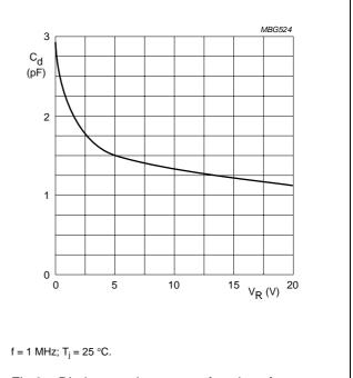
ent as a function of junction Fig.6 Diode capacitance as a function of reverse voltage; typical values.
