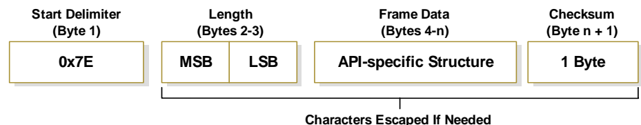
Figure 3-02. UART Data Frame Structure - with escape control characters:
