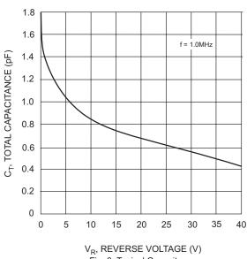
Fig. 3 Typical Capacitance
