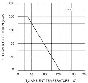
Fig. 4 Power Derating Curve, Total Package
