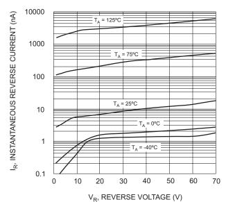
Fig. 2 Typical Reverse Characteristics
