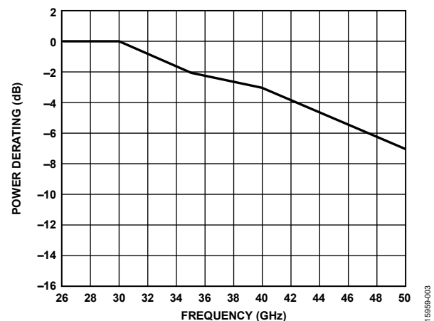
Figure 3. Power Derating vs. Frequency, High Frequency Detail, T CASE = 85°C
