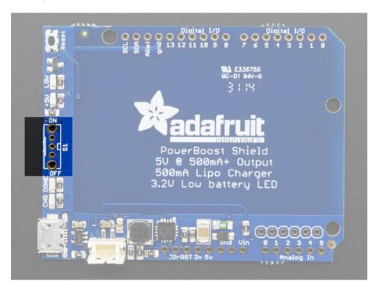
If you would like to custom attach your own switch, solder a switch to the middle pin and the pin right below the middle pin. Any voltage/current rating is fine as the switch is signal, not power, carrying
