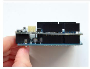
Start by placing the shield on top of an Arduino (any will do) and threading the four long stacking headers through so they plug into the Arduino headers.
