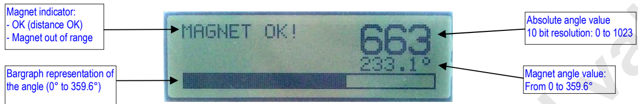
Figure 2: LCD display in standalone mode (9V battery or USB powered without GUI)
