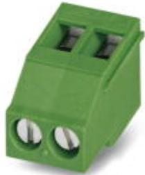
PCB terminal block, nominal current: 24 A, nom. voltage: 400 V, pitch: 5 mm, number of positions: 10, connection method: Screw connection with tension sleeve, mounting: Wave soldering, conductor/PCB connection direction: 90 °, color: green. The article can be aligned to create different nos. of positions!
