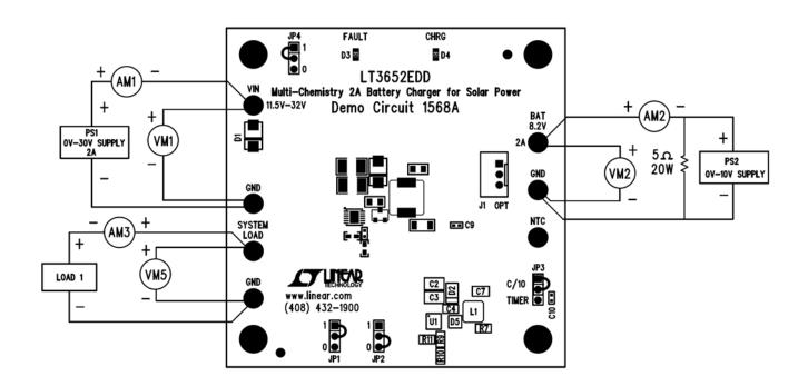
Figure 1. Proper Measurement Equipment Setup for the DC1568A
