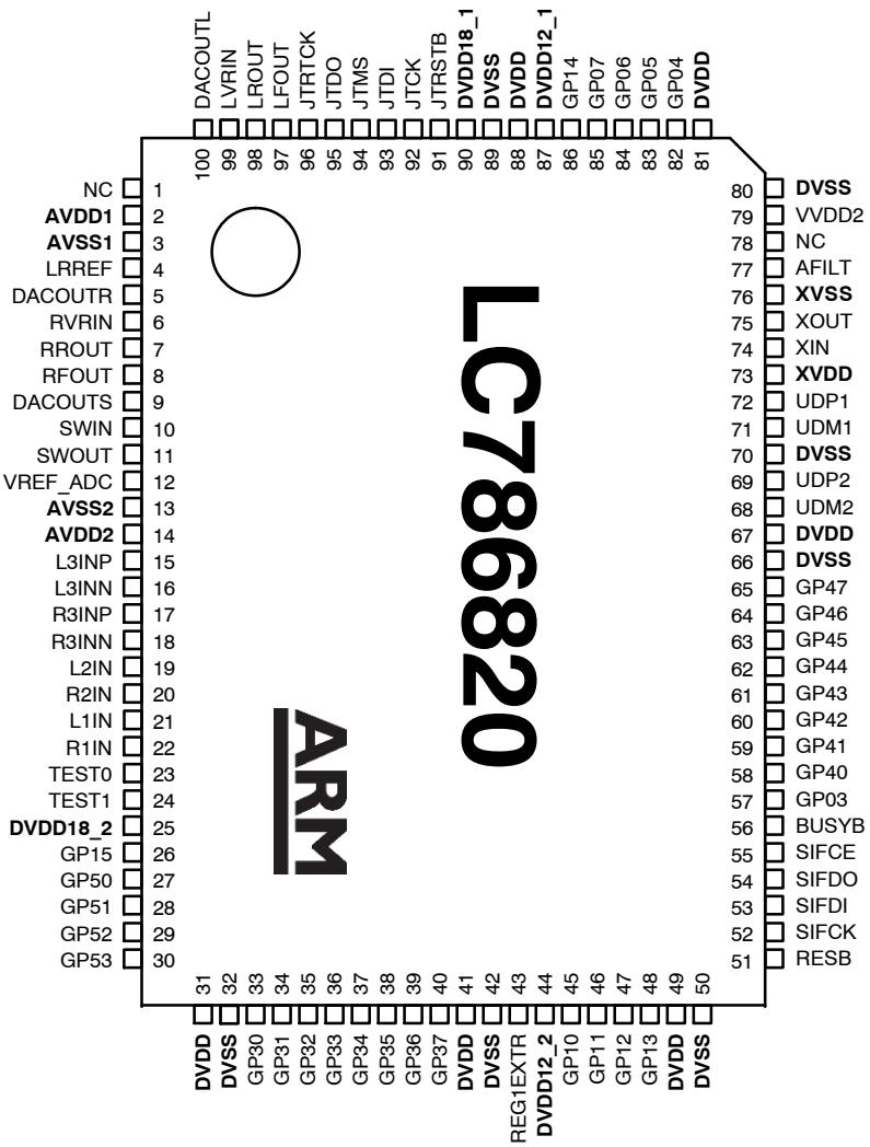
Figure 1. Pin Assignment
